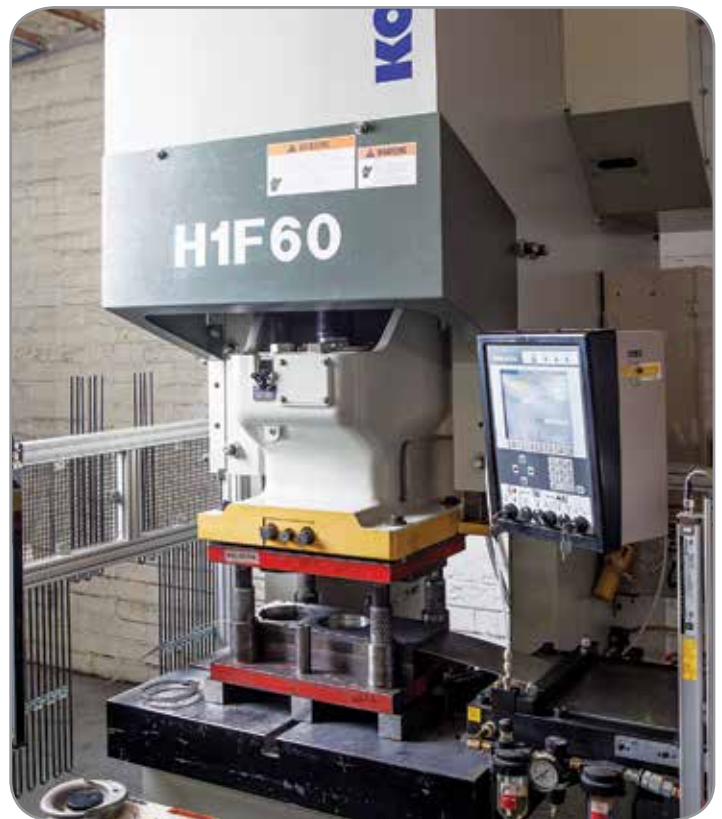
High Capacity Punch Press with Compound Hard Tool
